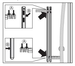
Secure the transit bars to the back of the washing machine. Make sure that holes ® are fitted over retainers A. The washing machine must not be moved without the transit bars in place.
